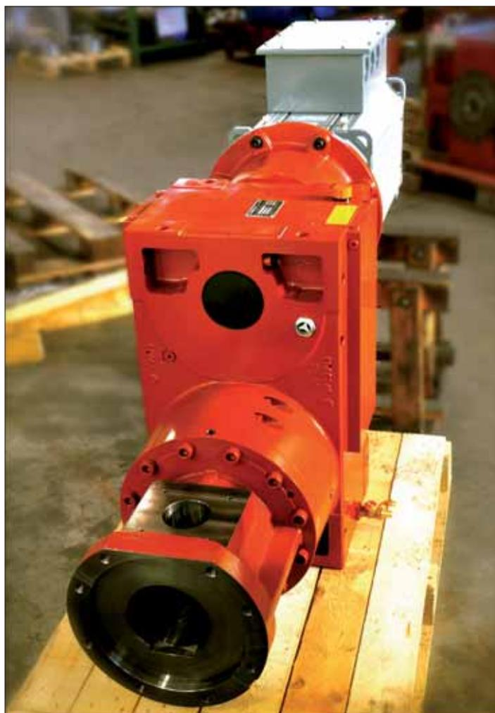
Gearmotor with feeding flange, for Single Screw Extruder
